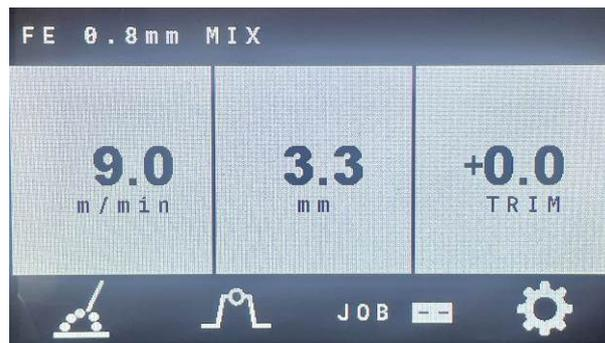
Once you select a program, the program is displayed . The top line in the display shows the name of the program, the wire diameter, and the required gas/gas mixture. The line below displays, starting from the left, the wire speed, material thickness and arc trim.
