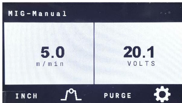
Turn left encoder ( Fig.4,ref. 16 ) to set the wire feed speed and turn right encoder ( Fig.4,ref. 12 ) to set the voltage. Press the button INCH ( Fig.4,ref.8 ) to momentarily feed welding wire at speed set without energizing welding circuit or shielding gas valve. Press the button PURGE to flow gas and purge air from gun or adjust gas regulator. These two functions are available only in MIG MANUAL MODE.
