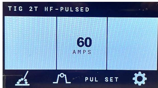
For regulate the pulse parameters press the button PUL SET ( Fig.4,ref. 10 ) . With the encoder ( Fig.4,ref. 12 ) you can regulate the value of the Frequency ( Hz ) . The value is adjustable from 0,4 to 1000 Hz .
