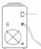
The Inverter TIG µP 403H DC is supplied equipped with a coupling for connection to the A.W.C. water cooler.
