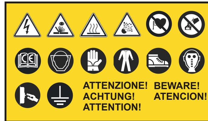
SAFETY SIGNS FOR WELDING MACHINES – IN COMPLIANCE WITH DIRECTIVE 92/58/EEC AND WITH STANDARDS UNI 7543-1-3
