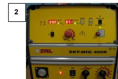
Press, at the same time together, for 3 seconds PURGE (C) and INCH (D) buttons.
