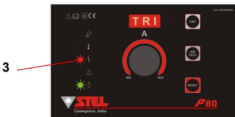
1. The operator Turn ON the unit with the torch trigger pressed or broken.
