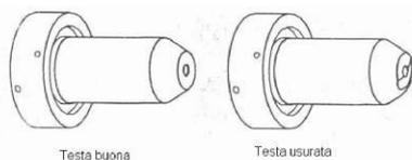
4. Remove the starter cartridge. Check for excessive wear plugged gas holes, or discoloration. Check the lower end fittings for free motion. Replace if necessary.
